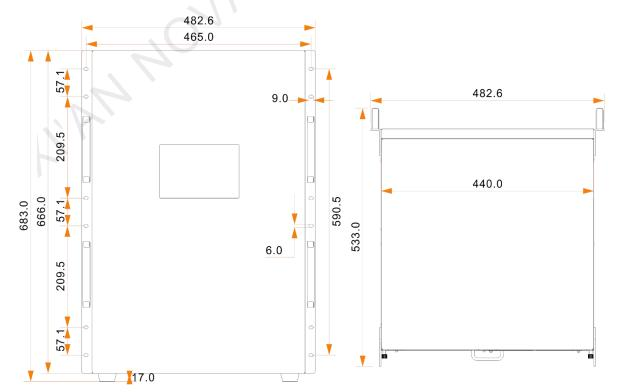
Tolerance: ±0.5 Unit: mm
